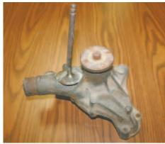
Magna 777 rod provides machinable welds that won't crack on most types of cast iron. Photo shows a steel valve welded to a cast iron pump.
