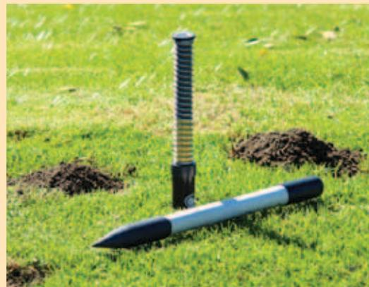
The GopherHawk trap kills gophers and moles immediately without the use of poisons or bait (left). The three-pronged, stainless steel snare and trigger are exposed in the tunnel when the trap is engaged (above left). A probe and wedge tool is used to find the tunnel and make a hole into it (the thin probe stores inside the wedge). Then the trap is inserted in the hole vertically. The yellow stripe indicates the trap has been triggered (above).
