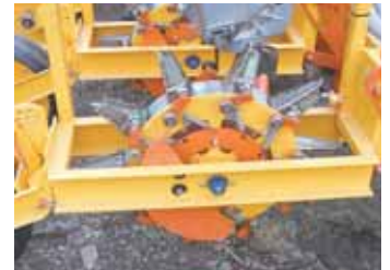
Polyplanter lays plastic over beds and opens up holes for seeds, then plants into them. Circular planting head has up to 15 removable points and a variety of seed plates.
