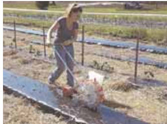
Ferris Farm also makes the Polyplanter Junior, a mini seeder that can be used by one person. You can plant seeds as small as lettuce and as large as lima beans. Comes with 10 seed discs that allow you to adjust spacing in the row. Current model is being phased out. New model of mini seeder will be out by August, 2017.
