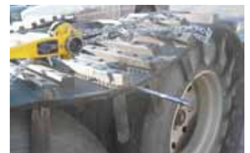
Photos show how ends of track are joined together using a come-along to insert a steel rod through interlocking teeth.
