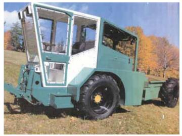
Maury Collins's PRO III 4-WD articulated tractor is powered by a 90 hp. Deere diesel engine. Tractor's rear half is available for use as a flatbed, dump box or log bed.
