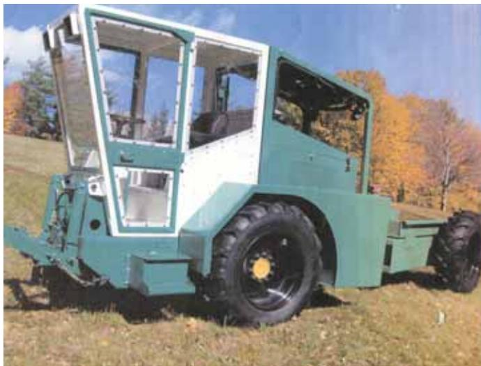
Maury Collins's PRO III 4-WD articulated tractor is powered by a 90 hp. Deere diesel engine. Tractor's rear half is available for use as a flatbed, dump box or log bed.
