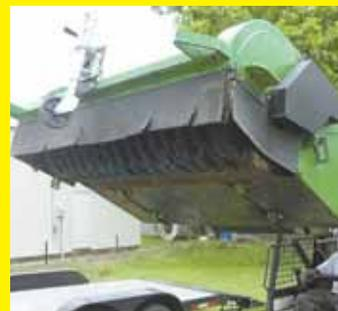
I used to watch city workers with rakes and shovels cleaning the edges along sidewalks and then running a sweeper over them. I figured there had to be a better way so I built my new skid loader-mounted Edge Master power sweeper, which is designed to edge and sweep in a single pass. It can clean and edge 100 ft. of sidewalk in less than 2 min.
