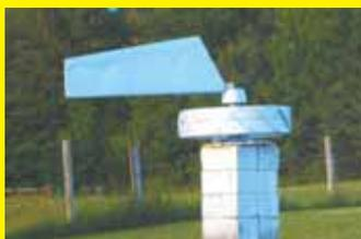
I made a big wind direction finder for my yard that's easy to see. I mounted a steel drive wheel from an old binder - complete with bearings - on top of a pillar of blocks, and then attached an
