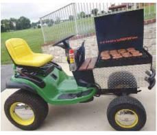
Dale Clugston's barbeque grill mounts in place of the engine on his Deere lawn tractor. Power to move the mower is supplied by a 12-volt electric motor.
