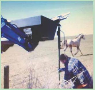
Tee-Post driver hangs from loader bucket. Post slips into driver barrel, which swings freely on swivel, allowing gravity to align posts. A post puller attachment is available that consists of a pin that locks onto fence post notch so that posts can be pulled quickly with driver.
