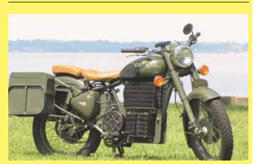
My Royal Enfield Bullet 500 motorcycle had a blown engine, so I had to do something. I decided to convert it to electric so it's now powered by a Motenergy ME1003 permanent magnet DC electric motor that goes where the transmission was and is located in front of the swing arm. Two stacks of batteries fill in the space where the engine used to be. They consist of 11 lithium battery modules taken from a Nissan Leaf electric car (the Leaf uses 48 modules).
