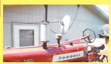
I mounted a mirror on the hood of an old yard tractor that we primarily use to move and spot trailers. Saves a lot of time lining up and it saves you from continually twisting to look back. It also helps keep an eye out for grandkids. Another tip is that I use a smaller 2-in. ball for hooking up to 2 5/16 ball hitches when moving trailers just a short distance. Makes it easier to connect. (Gary Swensen, Yankton, S. Dak.)
