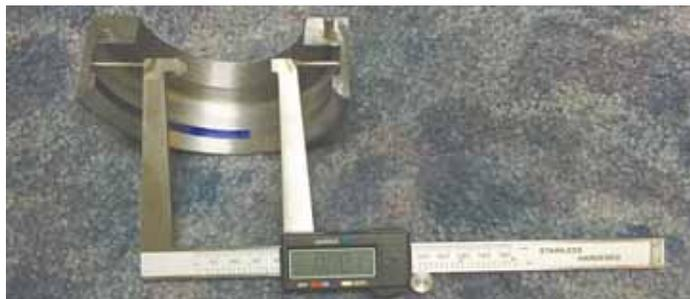
**Paxton's "made it myself" measuring tool solved the problem of measuring the "stepped bore" design of a housing he was machining.**
