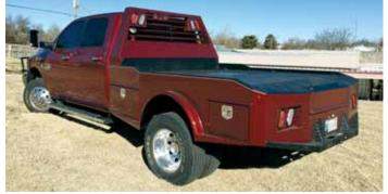
Schmidt's standard flatbed includes a steel floor, custom headache rack, 4 under-thebed toolboxes, LED lights in the window, and a rear bumper.
