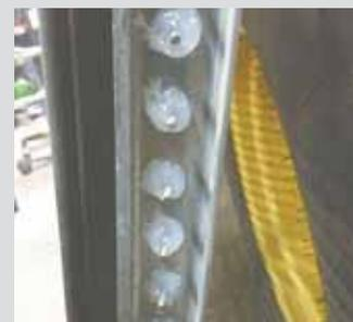
Photo shows worn sieve wires that Gutschmidt cut off with a Dremel tool. He welded new wire stock in place and then silenced the ends to stop the wires from shaking.
