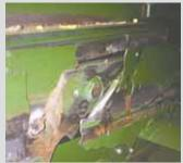
Photo above shows damage that occurred when lower sieve broke away from sidewall. Had the angle iron support holding it up been welded on the top side (as shown below), the breakage would not have occurred, says Gutschmidt.
