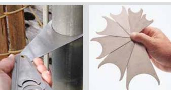
Tool consists of 7 riveted-together "sizers" that you fit over pipes to be measured.
