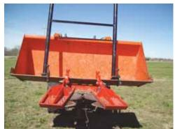
by clamping the cutting assembly and metal guard onto the lip of the bucket, using special mounting brackets. Or, you can chain the cutting assembly to a clevis attached to a bracket that's clamped onto the bucket. The ATV frame that supports the cutting assembly runs under the loader and attaches to the tractor's front end. "Raising the bucket gives you a better view of the cutting assembly."
