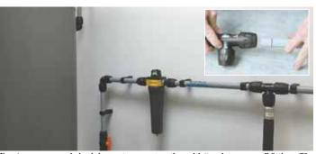
DanAm compressed air piping system goes together with "push to connect" fittings. The modular design uses reinforced nylon couplers (inset) to connect runs of pipe together, making it easy to assemble, change and expand.
