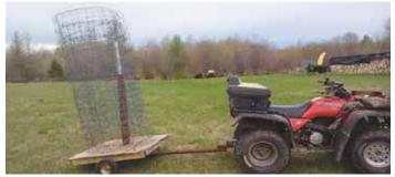
Atv-pulled, trailer-mounted fence unroller makes unwinding rolls of woven wire fencing an easy job for Rolland Girard of Cochrane, Ontario.
