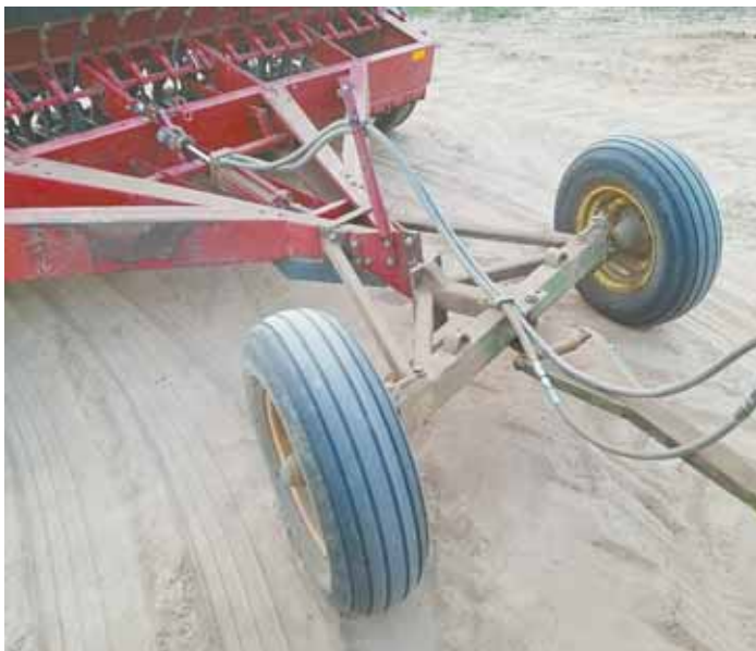
Photo shows bracket connecting drill hitch to running gear axle.
