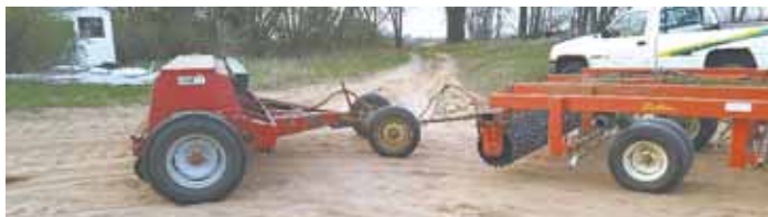
To keep the drill level, Derrick's dad attached the steerable front axle of a Deere 1065 running gear to the drill.
