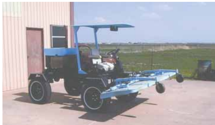
He fabricated a cowl for the engine and a canopy over the driver's seat. A hydraulic cylinder is used to control mower's cutting height.
