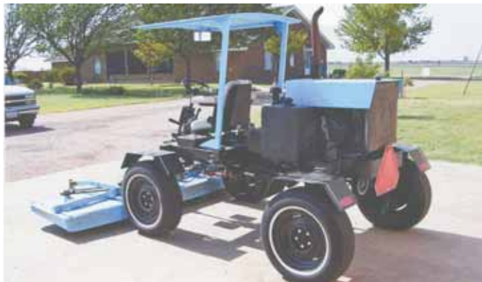
Daryl Dixon converted an old Schweiss self-propelled spot sprayer into this 8-ft. mower, reducing machine's height by 2 ft. and bringing the wheels in for a 6-ft. width.
