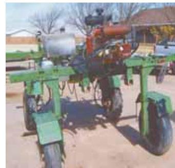
Sprayer's 8 hp. Kohler engine was replaced with a 30 hp. diesel mounted on back of machine.
