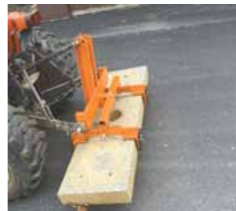
Home-built, 3-pt. mounted lift takes the back work out of leveling flat grave markers. It's adjustable for headstones from 16 to 24 in. wide.
