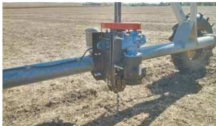
Pivot Guard drills an auger bit 4 ft. into the ground to help keep center pivots from rolling over in high winds.
