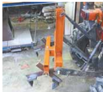
Home-built, 3-pt. mounted lift takes the back work out of leveling flat grave markers. It's adjustable for headstones from 16 to 24 in. wide.
