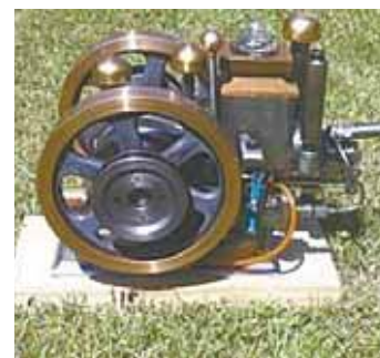
Tiny “hit and miss” diesel engine measures 12 by 18 in. and is 14 in. tall.
