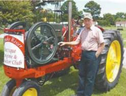
Tom Shell replaced the engine on his Massey Harris 30 tractor with a McCormick-Deering "hit and miss" engine. It powers a hydraulic pump that runs a hydrostatic motor mounted on the transmission
