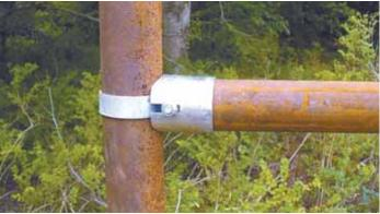
Pipe connector kit includes a band that clamps onto a 2 7/8-in. pipe post, and a double-slotted sleeve that slides over a 2 3/8-in. cross pipe. A carriage bolt runs through band.
