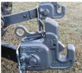
**Dean Weatherly, Clinton, Ark.:** Dean's pleased with his **Pat's Easy Change** 3-pt. hitch system (www.pats3pointhitchsystem. com; ph 850 398-8453). The units mount on your tractor's 3-pt. lift arms and turns them into quick hitches, making it easy to attach heavy 3-pt. implements without any lifting. The 3-pt. top link is still able to flex and float and your 3-pt. can be used normally.
