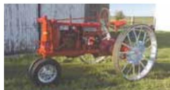
wheeled tractor as his "best buy." "I bought the F-12 for parts to use on a Farmall F-14 that I was restoring. However, once I got the F-12 home and started working on it I realized I could fix it up cheaper and easier than the F-14. After rebuilding the carburetor and replacing the magneto, I was able to get the F-12 started. I spent the following winter and early spring restoring this tractor to its former glory."
