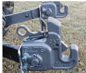
**Dean Weatherly, Clinton, Ark.:** Dean's pleased with his Pat's Easy Change 3-pt. hitch system ([www.pats3pointhitchsystem.com](http://www.pats3pointhitchsystem.com); ph 850 398-8453). The units mount on your tractor's 3-pt. lift arms and turns them into quick hitches, making it easy to attach heavy 3-pt. implements without any lifting. The 3-pt. top link is still able to flex and float and your 3-pt. can be used normally.
