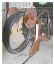
One-row "plow" is used to place 1-in. plastic water line underground.
