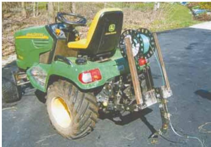
"It works on the same principle as machines that install drain tile in farm fields," says Don Myers about the 3-pt. mounted cable layer he built for his lawn tractor.
