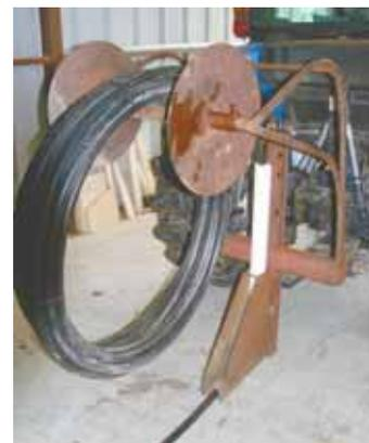
One-row "plow" is used to place 1-in. plastic water line underground.
