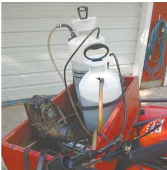
Alan Linda connected an old Black & Decker 12-volt compressor to a pair of spot sprayers, eliminating the need for hand pumping.
