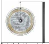
Nut hanging freely from string bangs against aluminum pie plate as plate flaps around in the wind
