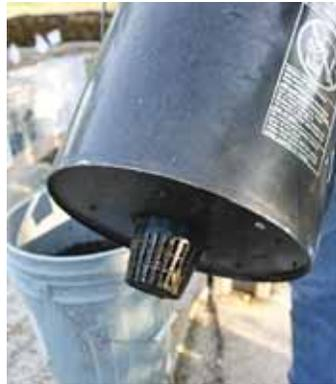
Plastic net filter cup is inserted into hole cut into bottom of each bucket, to draw water out of rain gutters.
