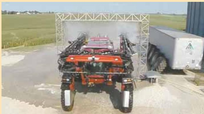
Nozzles positioned at opposing 35-degree angles blasts equipment as it passes through. Separate nozzles at ground level direct water up and under machine.
