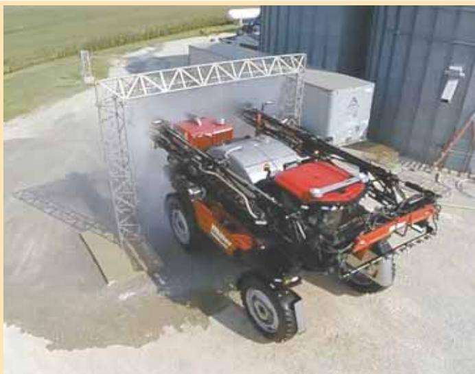
Neil Welsh keeps his self-propelled sprayer clean with this drive-thru equipment washer. Pipe framework bolts to large concrete slabs on either side.
