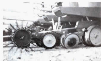
New-style harrow has 36 pairs of steel teeth per unit. Depth is controlled by guide wheels ahead of the teeth.
