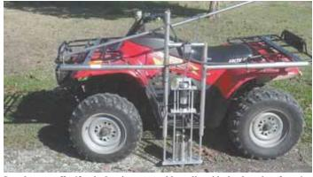
Sampler runs off a 12-volt electric motor and has adjustable depth settings from 4 to 10 in. "You manually control how fast you take the sample," says Mike Machek.
