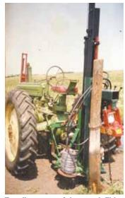
To pull posts out of the ground, Fisher hooks a chain to a sleeve on the mast that holds the auger.
