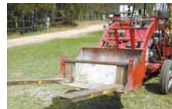
Halaska also fabricated a set of forklifts for the tractor's loader. "When I don't need the forks, I just tip them back to a stand on top of the bucket and tie them down," he says.
