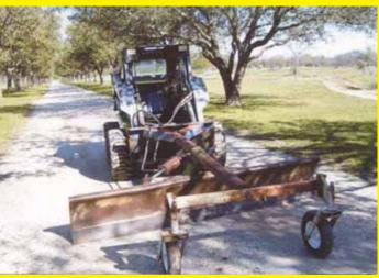
Here's a photo of a skid loader-mounted road grader that I built out of scrap materials
