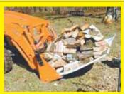
I made this bucket extender for my frontend loader from a scrap car hood and some old chains. The hood slips into the loader bucket and a chain runs from the top of the bucket to the outer corner of each side of the hood. It's great for carrying wood and other bulky loads. (Frank Heraghty, Claremore, Okla. (ph 918 342-5809)
