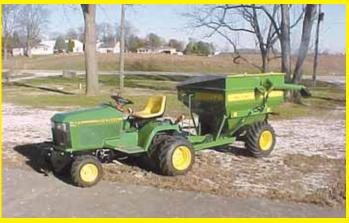
I built a grain cart to pull behind a John Deere garden tractor that has a 540 pto hothit a grain cart to pun behind a 30im Declind a grain gate on the auger opens and closes by hydraulics and the auger also folds up and down with a hydraulic cylinder. It also has a hand-rolling tarp. I also put dual wheels on the garden tractor. I've gotten many nice compliments on this setup. (Bruce Nickel, 1477 Goodpasture Rd., Concord, III. 62631; pdn74@hotmail.com)
