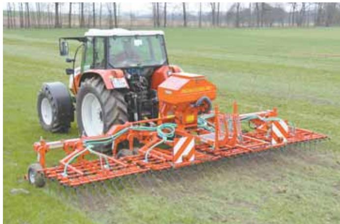
**Einböck tined seeder loosens the soil and evenly deposits seed across its 20-ft. width using pneumatic tubes.**
