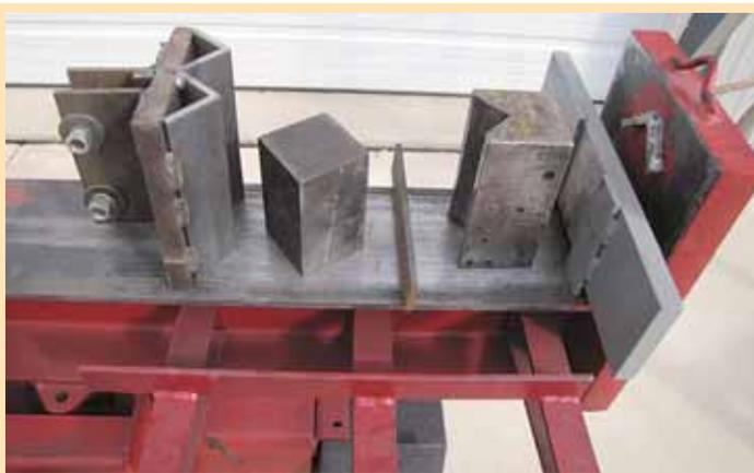
To convert his log splitter to bend steel, Gruenberger drilled 2 holes in the wedge and then bolted a homemade head onto it. He also fabricated a square steel block and a 90-degree V-block.
