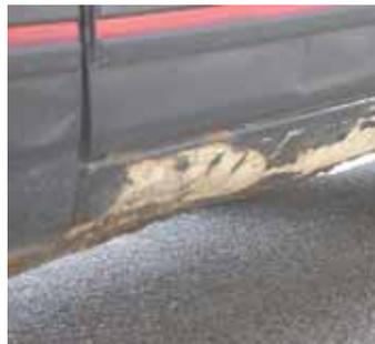
Bob Halaska filled in rusted areas on his 1975 Jeep Cherokee with spray foam insulation to keep moisture away. Photos show where he covered vehicle's underside.
