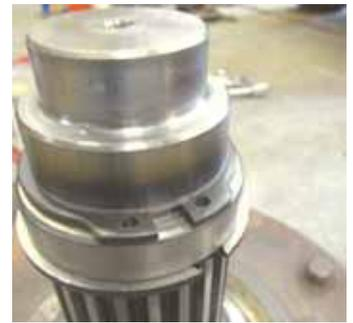
**To keep snap ring from coming loose, Strawhacker added a second ring inside the original one and used a tapered bearing cone as a hardened spacer.**
