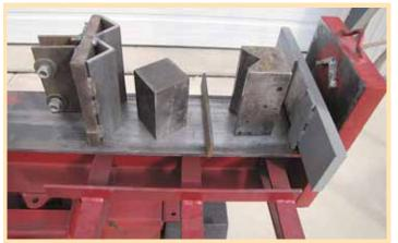
To convert his log splitter to bend steel, Gruenberger drilled 2 holes in the wedge and then bolted a homemade head onto it. He also fabricated a square steel block and a 90-degree V-block.
