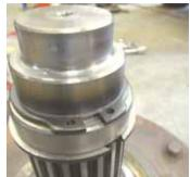
To keep snap ring from coming loose, Strawhacker added a second ring inside the original one and used a tapered bearing cone as a hardened spacer.
