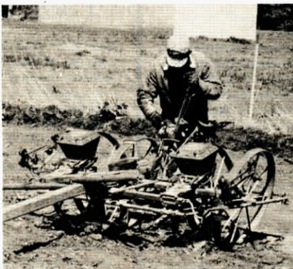
One of five strikes against Deere's BRASS/HANSEN patent on the Max-Emerge was that the canted furrow-closing wheels, claimed to be new invention, weren't new. The old Hayes No. 44 planter, popular in the 1930's, had canted wheels to provide, as the manufacturer points out in a 1935 manual on the planter... "a firm seedbed. The pressure of the wheels set on an angle firms the soil in a V-shape with the seed. This puts the seed in close contact with moist soil for quick germination..."
