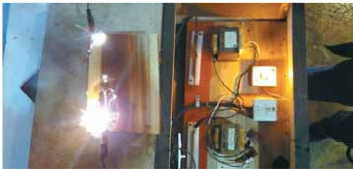
Dave Fox made 2 burners that he uses individually or in tandem to create art. One is made from a microwave oven transformer.
