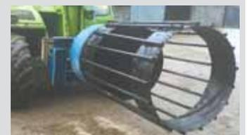
Rotating "stone barrel" scoops up rocks and then rotates hydraulically, allowing dirt to fall back onto field.
