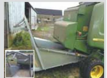
Hydraulically-operated accumulator leaves pairs of bales across the field.
