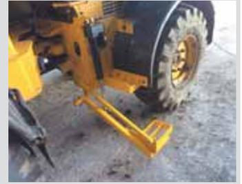
Replacement step lifts Bell up to his tractor cab hydraulically.
