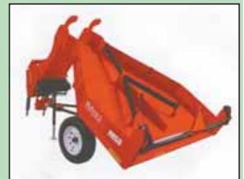
support a floor that’s permanently mounted at a 45 degree angle. A twisted chute mounts on front of the machine and hooks up to the baler chamber. ([www.kuhnsmfg.com](http://www.kuhnsmfg.com); ph 877 296-5851)
