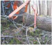
Log skidder has scissors tongs with 1-in. spikes, which grip log so it can be lifted by tractor 3-pt.
