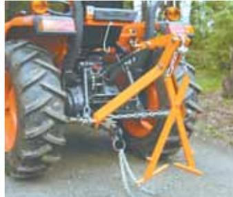
He fitted his 38 hp. Kubota tractor with a 3-pt. mounted log skidder that he invented.
