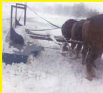
Thank you for your article a year ago on our dumping snow blade made out of a curved Harvestore silo panel. It's designed to be pulled by a 2 or 4-horse hitch and we've used it since 2010. Last spring we redesigned the tongue latching and unlatching system to improve operating efficiency. It lets anyone who doesn't have a skid steer or tractor snowblower clear a driveway easily using horses. (**Jesse Fisher, 347 School Lane Rd., Gap, Penn. 17527 ph 717 442-8958**)
