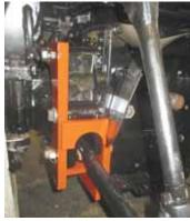
Bolt-on kit is designed to repair a broken rear axle housing on Deere 4000 series tractors. The problem happens when the pin hole for the 3-pt. lift arm breaks out of the axle housing.
