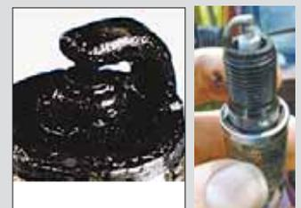
**Alan Linda, New York Mills, Minn.:** "I own a 1997 Chevrolet 1/2-ton pickup equipped with a 305 cu. in. V-8 engine, which was using a lot of oil – about a quart every 600 miles. The photo shows what
