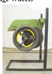
TR Solutions says its new "Mud Rx" keeps gauge wheels from packing with mud.
