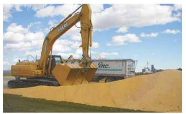
Massive 10-yard grain bucket mounts on an 80,000-lb. tracked excavator. It was built for a local elevator needing something big to load a half-million bu. of corn piled on a street.
