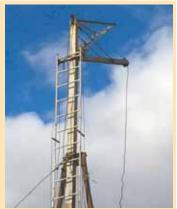
Ladder has an outrigger on top, which is used along with a hydraulic-operated winch and cable to lift heavy objects. Ladder is mounted on frame of an old auger.
