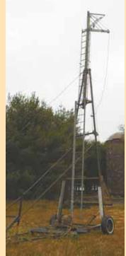
Bill Fluhrer built this hydraulic-operated ladder that reaches up to 35 ft. high. He uses his tractor to pull it around and also to operate the hydraulics.
