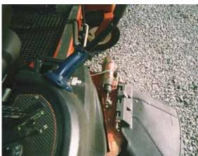
Cordless drill's body attaches to mower deck and handle bolts to mower fender. Wiring runs from handle to drill motor, and from there to mower's battery. A short cable connects deflector.
