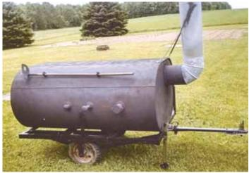
Rob Fetting built this portable burn barrel out of an old 100-gal. fuel tank that he mounted horizontally on a small 2-wheeled trailer.
