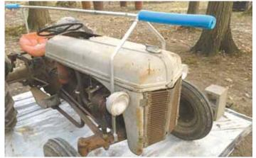
Pool noodles cut in half slip over front and back of frame to keep from tearing tarp.
