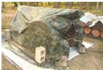
Mark Yax wanted to park his tractor in the woods for firewood hauling so he made a simple way to cover it, using a tarp that fits snugly over a tractor-mounted metal frame.
