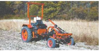
Oggun Tractor has modernized the old Allis Chalmers G tractor with independent hydraulic drive, steering, and lift. "Independent hydraulic drive allows zero-turn capability simply by stepping on one of the brake pedals," says Locky Catron.
