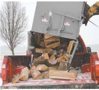
Bottom-unloading hopper lets you load firewood into a pickup or trailer bed without worrying about damaging the vehicle. Hopper slowly empties as it's raised.
