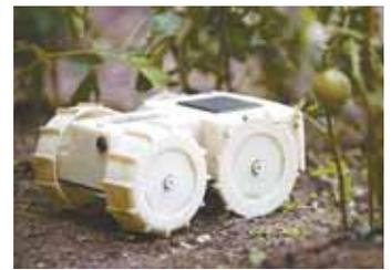
Equipped with a mini string trimmer, "Tertill" robot takes out newly emerged weeds in gardens. A sensor on front detects weed and activates trimmer, which is out of sight under body of robot.
