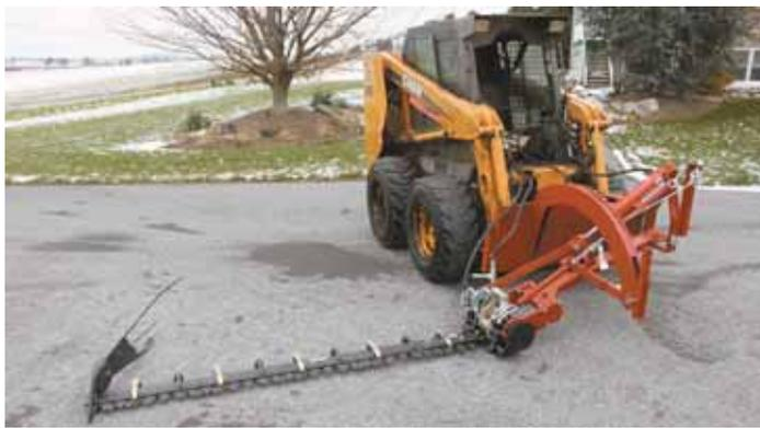
Front-mount sicklebar mower makes it easy to see what you're cutting. "Works great for cutting weeds and grass along pond edges and fences," says the company.
