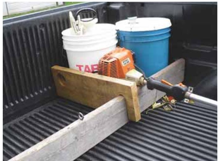
Slot cut into one end of a short 2 by 10 board hooks over a 2 by 6, forming a corner that keeps small items from sliding sideways.
